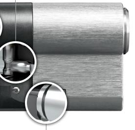
Rated break point In the event of a snapping attempt, the cylinder breaks at this rated break point.
